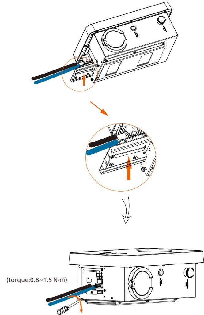
STEP 11: Push the rear cover to appropriate position of the cables and screw the self tapping screws with the cross screwdriver. Then tighten the waterproof fastening head.
