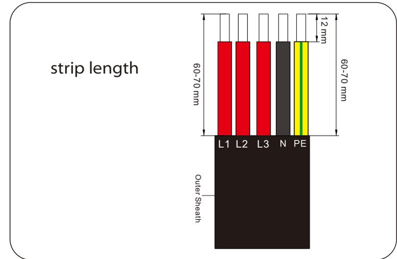
STEP 8: Insert the input cable through the waterproof connector in sequence as shown below.
