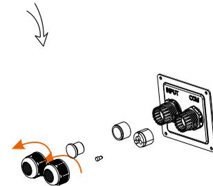
STEP 5: Unscrew the countersunk screw of the base plate of communication board with the cross screwdriver. Then pull the base plate of communication board out.
