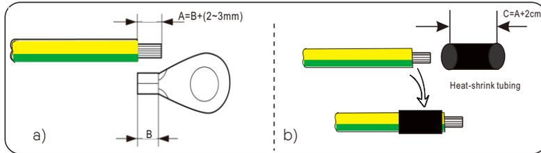
c) Insert the stripped section into the OT copper terminal and crimp with crimping tool.
