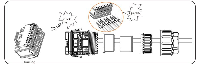
f) Push the seal body into seal ring, then push the claw.
