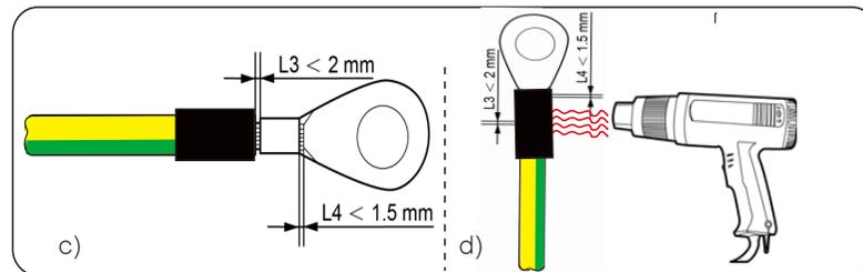
➤ Step 2: Connect the grounding cable to the inverter.
