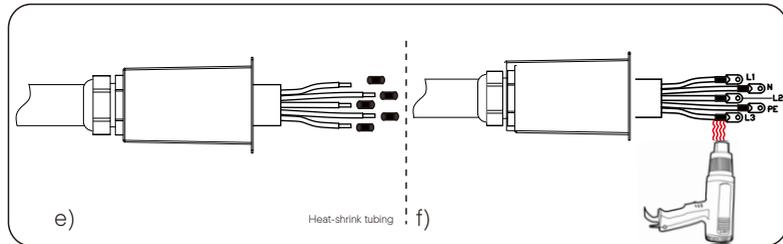
➤ Step 2: Connect the AC cable to the inverter
