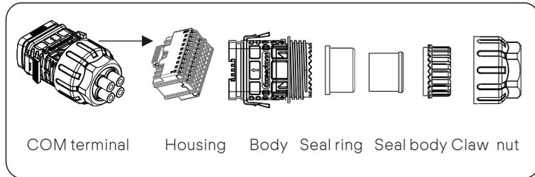
b) Select 0.5-0.75 mm<sup>2</sup> conductor and use wire stripper to strip 12-14 mm insulation layer of the cable end and insert the insulated cord end terminal to the cable end. (ENY0512 nylon terminal for 0.5 mm<sup>2</sup>/22 AWG conductor; ENY7512 nylon terminal for 0.75 mm<sup>2</sup>/20 AWG conductor)
