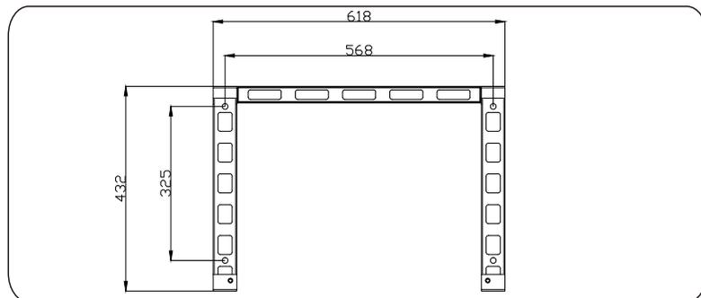
c) Use the bracket as a template for marking the position of drilling holes on the wall with a digital level and marker.
