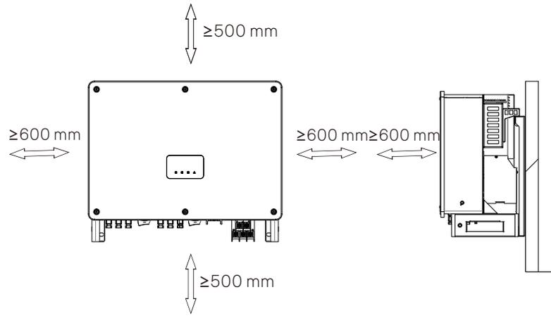
For multi-inverter installation, please reserve the space of 1200 mm at least between each left and right inverter and at least 500 mm between each upper and lower inverter.
